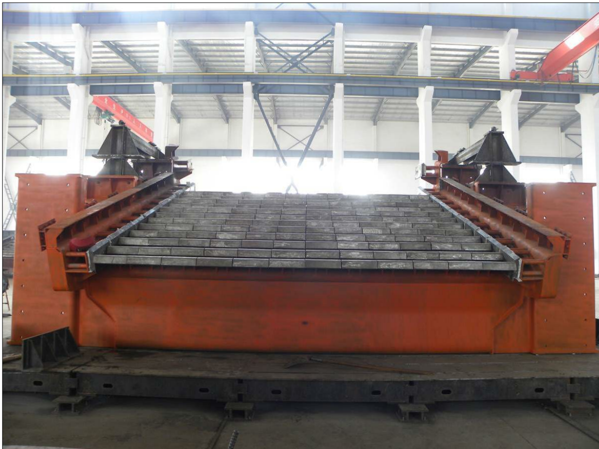
Figure 17: Section of furnace combustion grate
