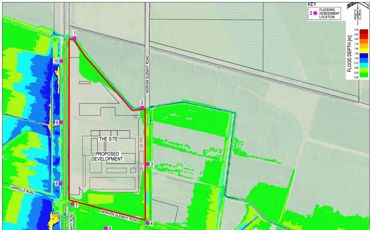
Figure 32: Post-development flood depth.
